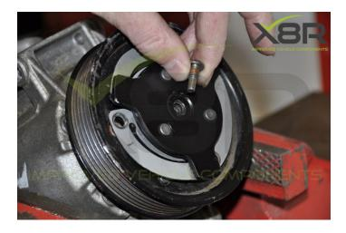
Step 2: Prise off the shear plate
