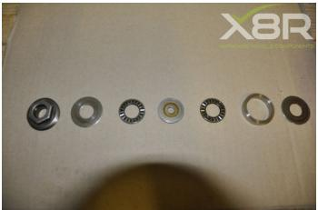
Step 9: Reinstall components with new outer ring Clean all bearing components and interior of piston (brake cleaner)
