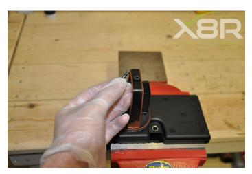
Step 3: Remove bell crank lever. Lift off cover on base of DISA unit.
