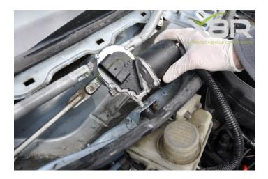
Step 8: Remove the old wiper rods
