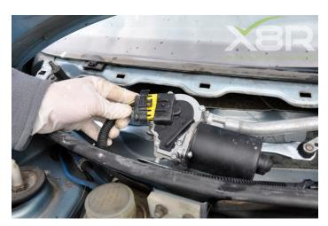
Step 7: Remove the wiper motor / linkage
