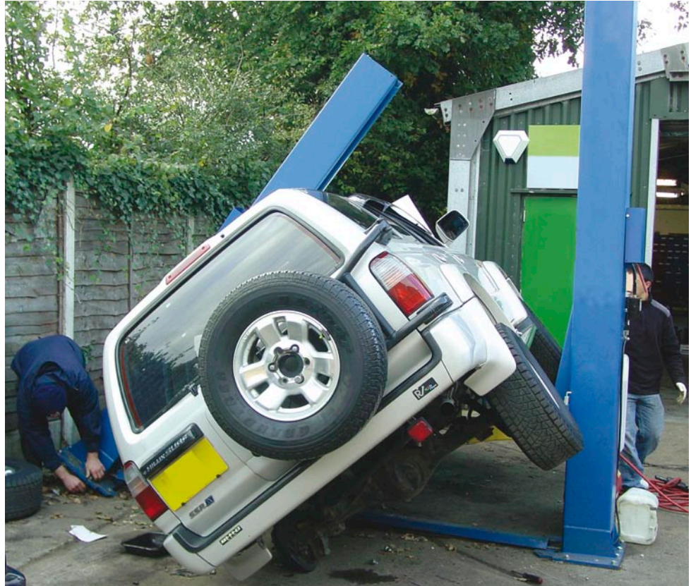
Figure 2 A collapsed two-post lift
