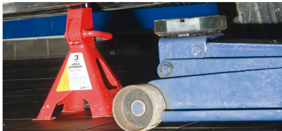
Figure 1 Car with trolley jack and axle stand on a firm, level surface
