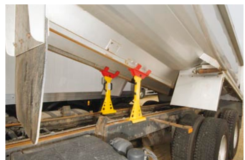
Figure 6 Props for a tipper lorry
