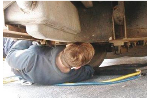
Figure 7 Limited clearance even with full suspension
