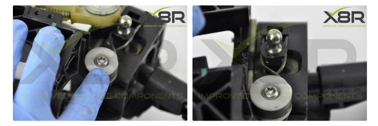
Mercedes Benz W639 Vito Viano Gear Selector Shift Stick Lever Bush Repair Fix Kit Manual Install Instructions Guide: Page 5
