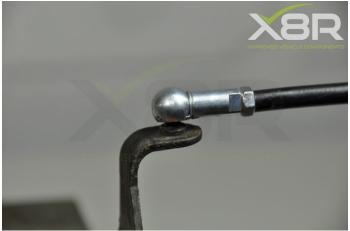
Step 7: Remove the two smaller rods
