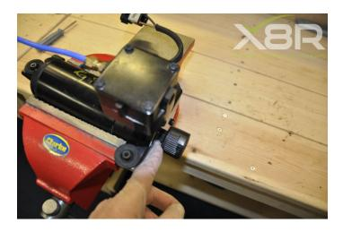
Step 2: Remove compressor head
