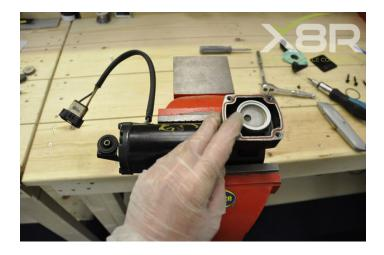
Step 7: Replace o-rings in head Remove two shims as shown.
