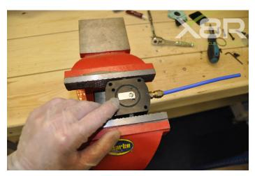
Step 8: Re-fit head and face plate and test. Apply Loctite to bolts and refit head.
