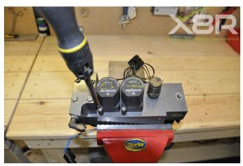
Step 3: Remove solenoid bases
