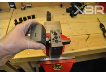
Step 6: Remove collets and O-rings Prise out collets with screw driver.
