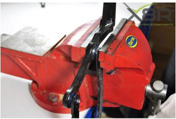
Step 13: Fit the bolt, washer and nut to retain the bearing The bolt can only be fitted one way as shown.
