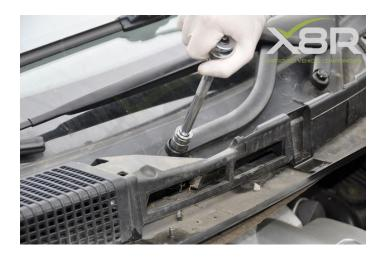
Step 5: Release the arms. Wind the nut back on a few threads.
