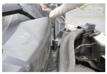
Step 3: Lever up and remove the scuttle panel Use a flat bladed screw driver to lever up the scuttle panel.
