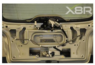
Step 2: Remove Lock Mechanism
