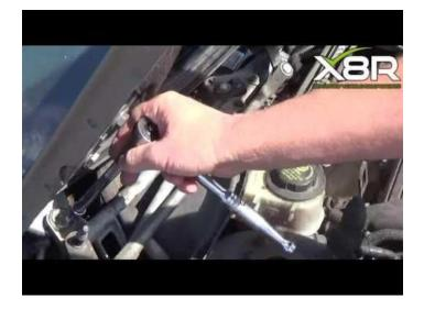
Step 1: Remove plastic spindle nut covers Lift bonnet and locate plastic covers on the end of each windscreen wiper.
