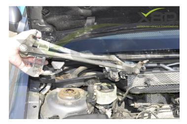
Step 6: Disconnect electrical connector Disconnect the electrical connector; to do so lever up the red plastic as shown and pull on the connector to release.
