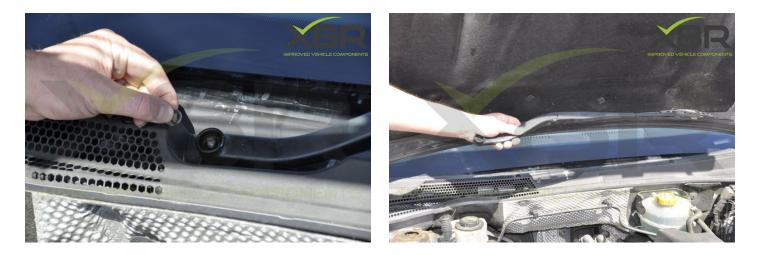
Step 4: Remove scuttle panel Remove the scuttle panel, this will bend in the middle to allow removal, the wiper jets are built in to the scuttle take care of the pipes, just move the scuttle to one side to allow access to the wiper linkage, there is no need to remove the scuttle completely.
