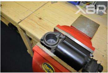
Step 3: Fit new piston seal
